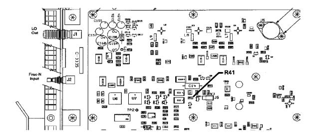
Unsolder A4R41 and replace it with the 162 ohm resistor. Use extreme caution since this is a surface mount component. Although probably not necessary, it is generally a good idea to redo adjustments #104 through #109. If the problem existed even when the analyzer was not in dither mode, then performing these adjustments is definitely required.
